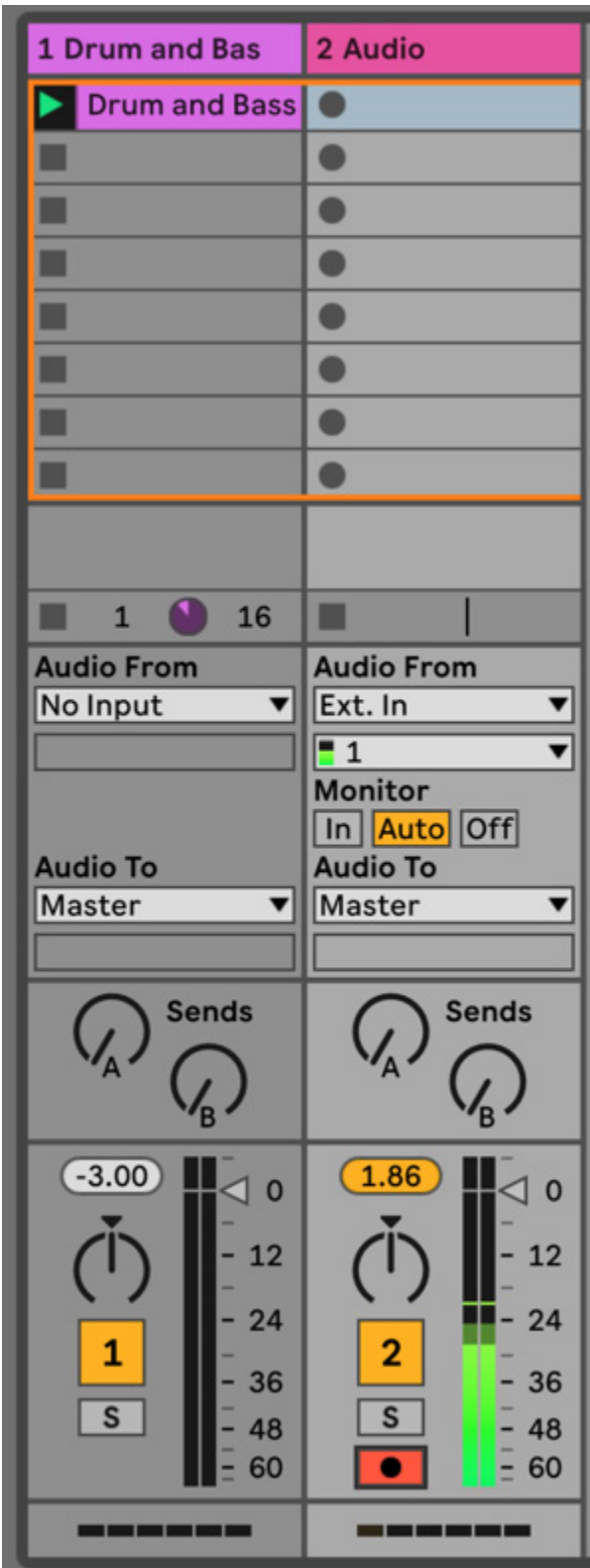
Figure 2.7 – The track is armed and an incoming signal is shown through the meter
