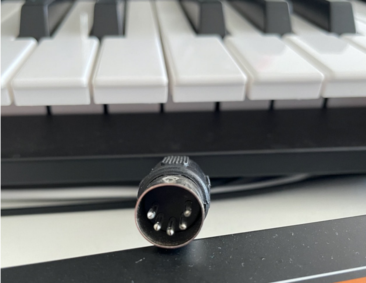
Figure 14.1 – Five-pin MIDI cable to send and receive MIDI information
